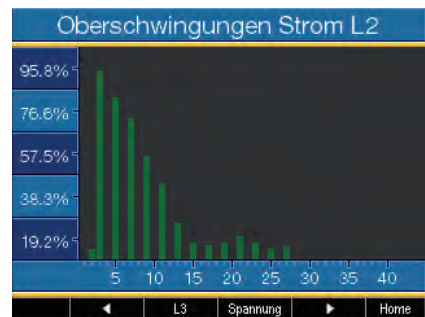
Fig.: Colour graphical display MRG 512-PRO PQ Flex – Example harmonics analysis
