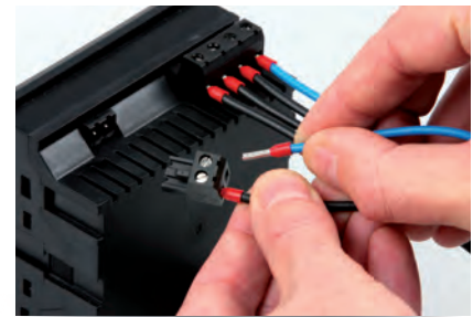
Fig.: Pluggable screw terminals for easy connection
