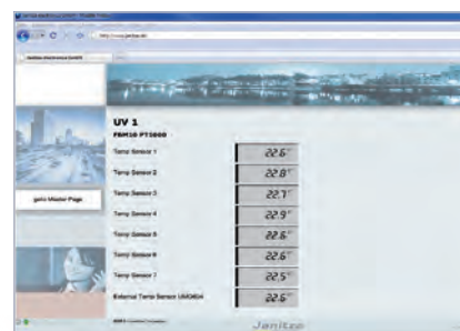
Fig.: Measured value display via the devices' homepage
