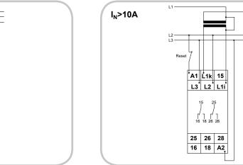
Connected to 3~ 400V mains with power module 400V AC and fault latch
