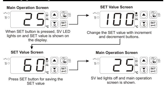
SET value is can be adjusted from minimum set value parameter  $5 \mu L$  to maximum set value parameter  $5 \mu H$ , Which can be accessed from programming parameters.
