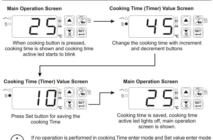
for 20 seconds, device turns to main operation screen automatically.
