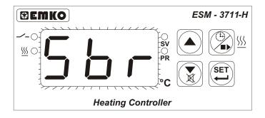
1- Probe failure in analog inputs. Sensor connection is wrong or there is no sensor connection. When this message is on the screen, if buzzer function selection parameter  $\fbox{buF}$  is 3 or 4, internal buzzer starts to operate.
