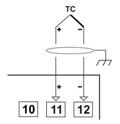
Connect the wires with the polarity as shown in the figure left.
