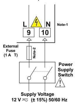
Note-1: "L" is (+), "N" is (-) for 12V === and 24V === Supply Voltage
