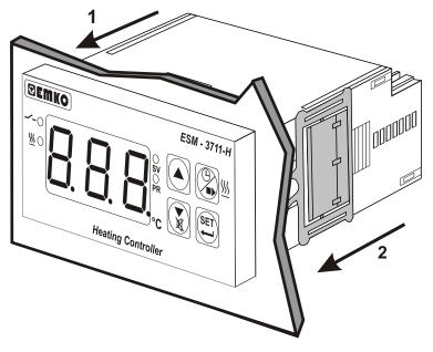
The unit is designed for panel mounting.
