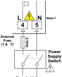
Supply Voltage 230 V ~ (± 15%) 50/60 Hz or 115 V ~ (± 15%) 50/60 Hz or 24 V ~ (± 15%) 50/60 Hz or 24 V ~ (-15%,+10%) 50/60 Hz
