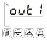
**5** - If user does not do anything for 120 seconds while device is on Set or Technician menus, device turns to operation screen.
