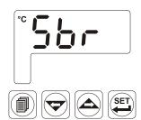
**1 -** Sensor failure in analogue inputs. Sensor connection is wrong or there is no sensor connection.
