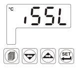
**4** - If technician password is different from "0" and user accesses to the parameter by Set button without entering the technician password and wants to change a parameter, the warning message is shown on display as shown on the left. Device does not allow to do any changes without entering the password correctly.
