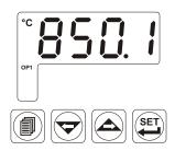
3 - If display blinks: If analogue input value is greater than maximum value of operating scale uPL, display starts to blink.
