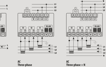
Attention: For the ADR-R E model the secondary circuits of the CT can not be earthed.
