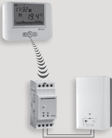
Example of connection with 1 channel remote actuator
