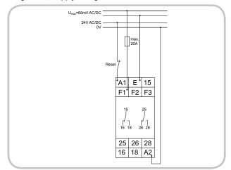
Range 150mV, supply voltage 24V AC/DC and fault latch
