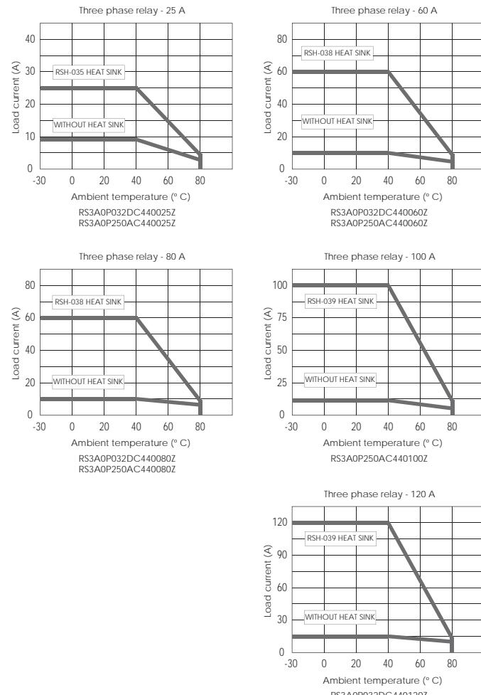
Over 10 A load a heat sink must be used. The use of a heat sink will make the lifetime of the relay up to four times longer, even when using it with load currents lower than 10 A.
