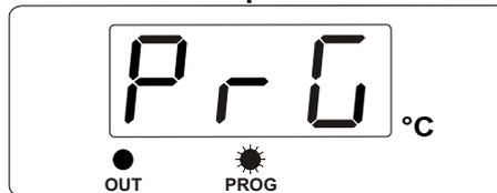
Press increment button for accessing to the password entering screen
