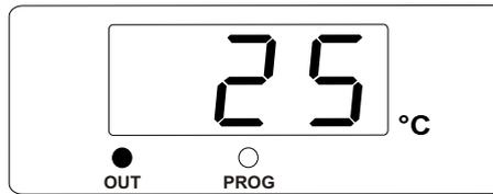
**Note:** If programming mode accessing password is 0, hysteresis screen **H51** is observed instead of **PrG** programming screen accessing password
