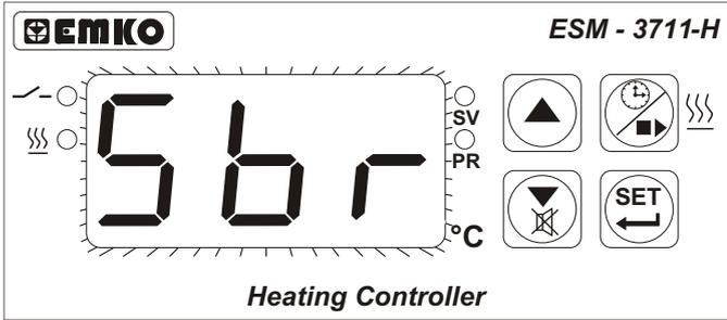
1- Probe failure in analog inputs. Sensor connection is wrong or there is no sensor connection. When this message is on the screen, if buzzer function selection parameter `b u F` is 3 or 4, internal buzzer starts to operate.
