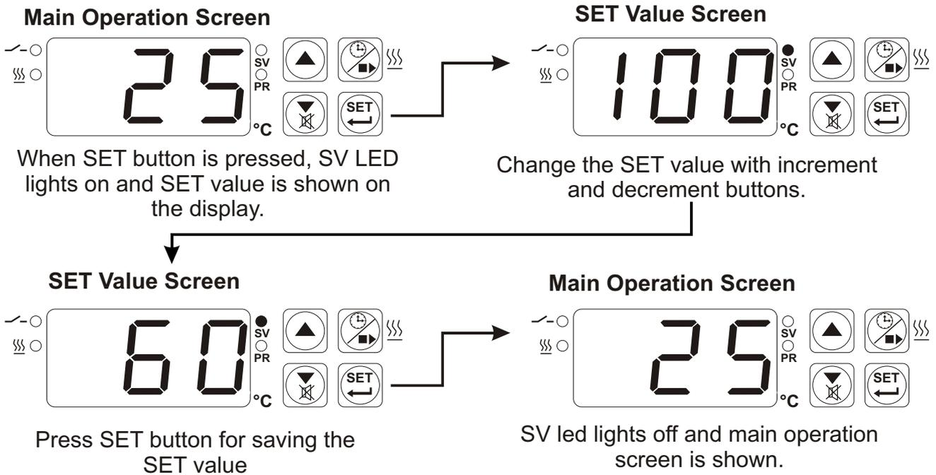
SET value is can be adjusted from minimum set value parameter **[5UL]** to maximum set value parameter **[5UH]** , Which can be accessed from programming parameters.
