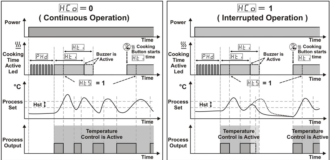
2- When cooking time parameter  $HE_1 = 1$ , if selection of temperature control and starting the cooking time parameter  $PHS = 1$  (Temperature control starts at power on. Cooking time (Timer) can be started by pressing cooking ON/OFF button or when cooking time start/stop input is getting closed condition) is selected;
