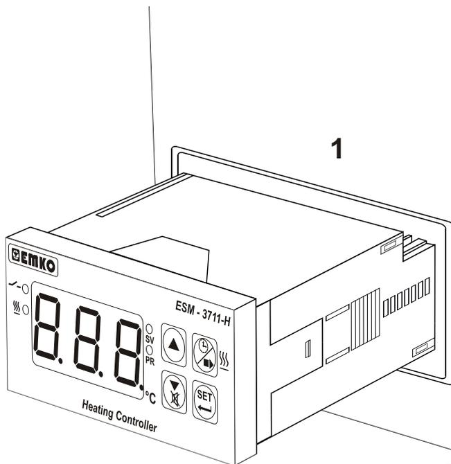
1-Before mounting the device in your panel, make sure that the cut-out is of the right size.
