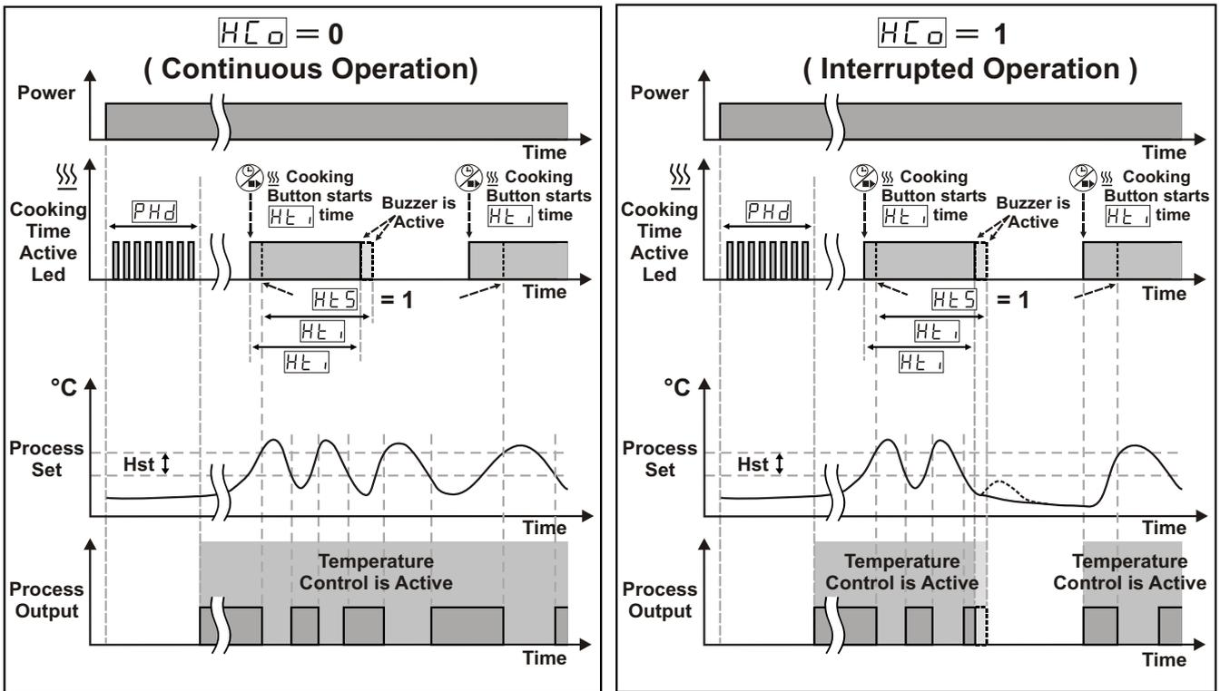
3- When cooking time parameter  $HE_1 = 1$ , if selection of temperature control and starting the cooking time parameter  $PHS = 2$  (Temperature control and cooking time (Timer) can be started by pressing cooking ON/OFF button or when cooking time start/stop input is getting closed condition) is selected;
