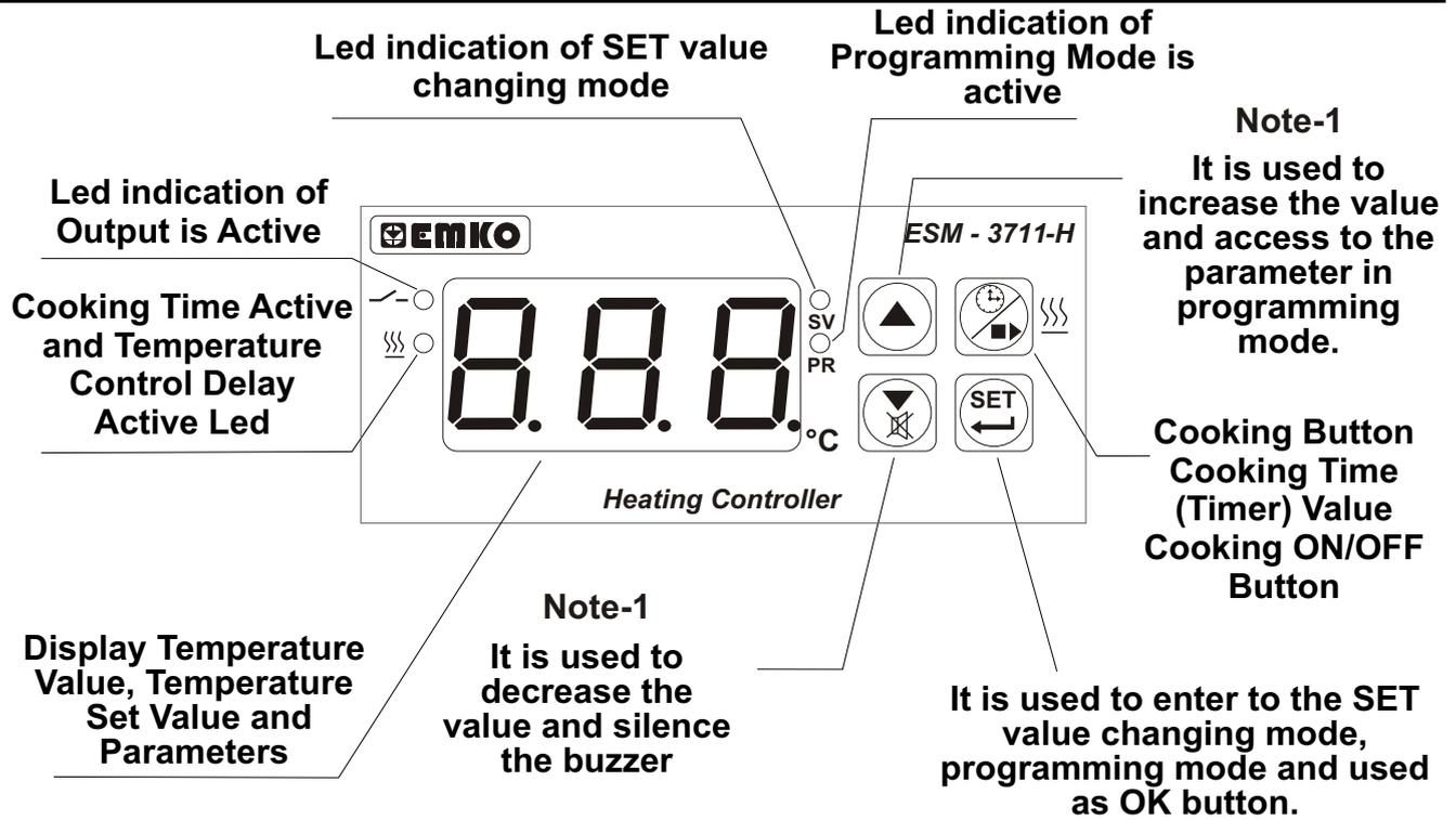
**Note-1:** If increment or decrement button is pressed for 5 seconds continuously, increment and decrement number become 10, if increment or decrement button is pressed for 10 seconds continuously, increment and decrement number become 100.
