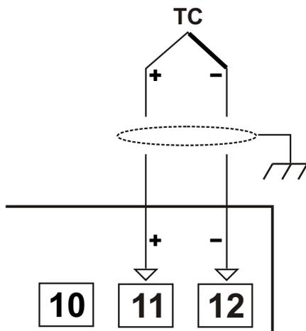
Connect the wires with the polarity as shown in the figure left.
