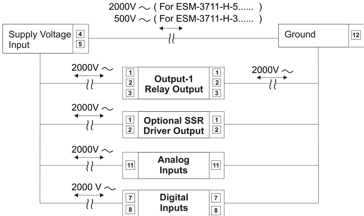
Galvanic Isolation Test Values for the devices with 12 V  $\approx$  Supply voltage input:
