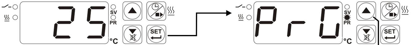
When SET button is pressed for 5 seconds, "PR" led starts to blink. If programming section entering password is different from 0, programming section entering screen **Pr 0** is observed.
