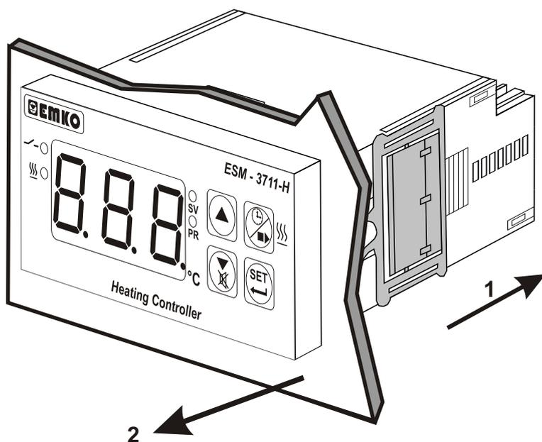
1-Pull mounting clamps from left and right fixing sockets.
