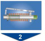
During this movement, the hydraulic fluid regulates the cores speed of travel, thereby creating a controlled time delay which is inversely proportional to the magnitude of the current.
