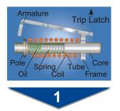
Hydraulic Magnetic Circuit Breakers (HMCB) operate on the magnetic force produced by a load current flowing through a series connected solenoid coil which is wound around an hermetically sealed tube containing an iron core, a spring and dampening fluid.
