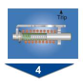
With high values of overloads or short circuit, the magnetic flux produced by the coil is sufficient to attract the armature to the pole face and trip the breaker even though the core has not moved. This is called the instantaneous trip region of the circuit breaker characteristic.
