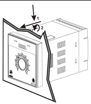
The unit is designed for panel mounting.
