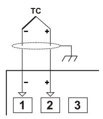
Connect the wires with the polarity as shown in the figure left.
