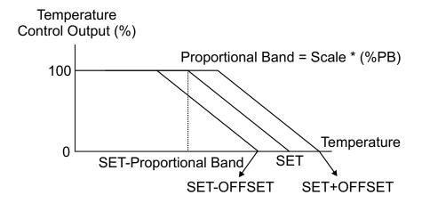
When temperature is not equal to SET value, to remove the difference between SET value and temperature and to make equal the temperature and SET value, set offset is used. It can be adjusted from -20% to 20% of full scale.
