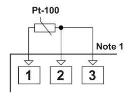
3-wire Pt-100 connection (with line compensation) (Max. Line impedance is 10 )
