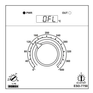
Sensor failure in analogue inputs.
