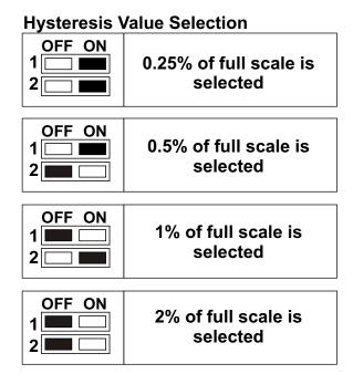
Minimum and maximum value of hysteresis according to the type and scale of the device are given below:
