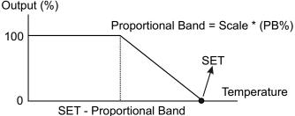
**Relay Output:** Output period must be short for stable process control. Relay must not be used in short output periods because of limited life of their relay contact (number of open/close events).
