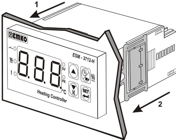
The unit is designed for panel mounting.
