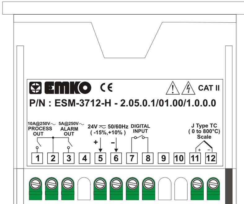
Device Label for J Type ( 0 ; 800 ) scaled, Thermocouple input, 24V  $\approx$  Supply Voltage Input and SSR Driver Outputs
