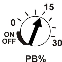
Trimpot is adjusted to point out different from ON/OFF part for proportional operation. Proportional Band Value can be adjusted from 0% to 30% of full scale.
