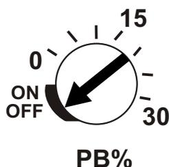
Trimpot is adjusted to point out ON/OFF part for ON/OFF Control form.
