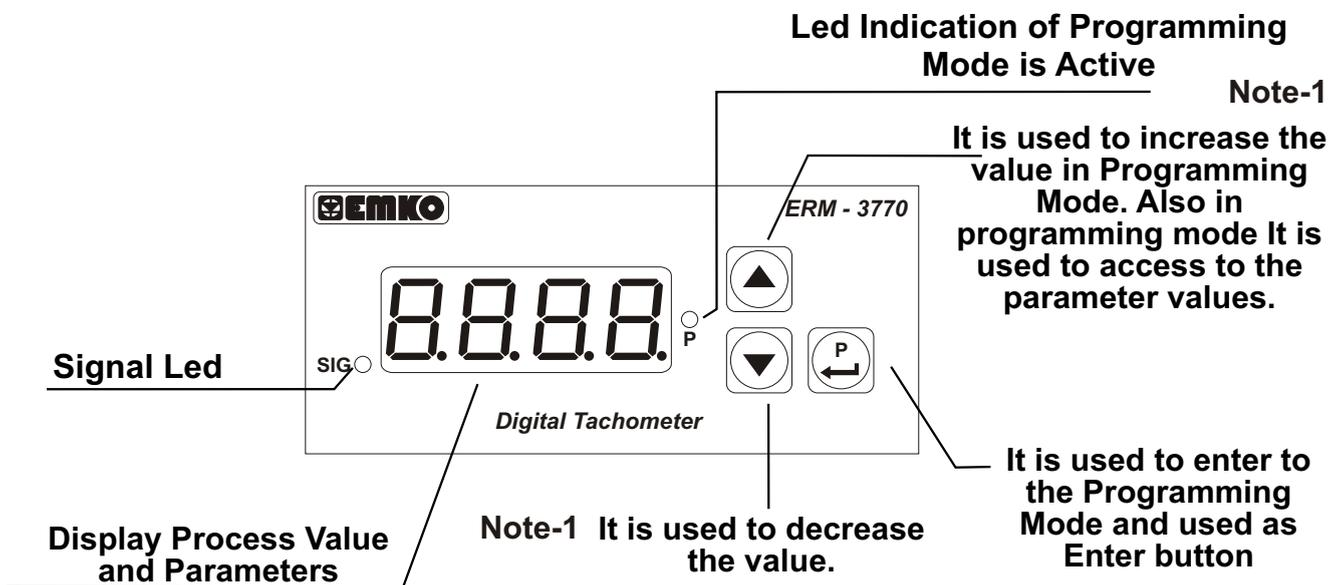
**Note-1:** If increment or decrement button is pressed for 5 seconds continuously, increment and decrement number become 10, if increment or decrement button is pressed for 10 seconds continuously, increment and decrement number become 100, if increment or decrement button is pressed for 15 seconds continuously, increment and decrement number become 1000.
