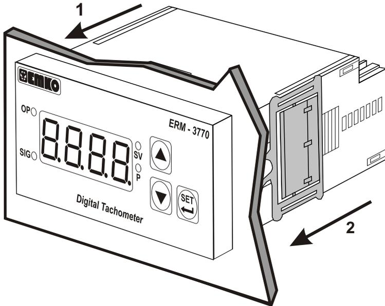
The unit is designed for panel mounting.
