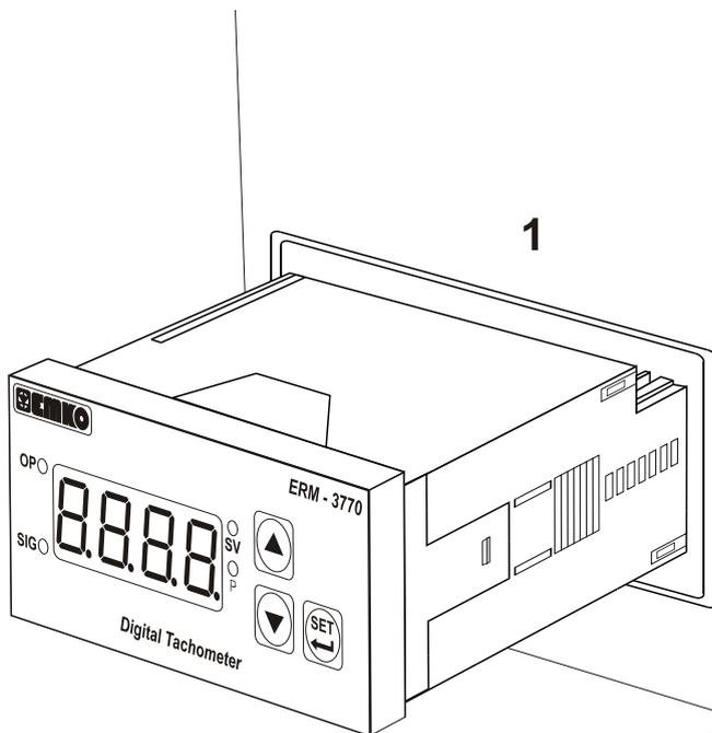
1-Before mounting the device in your panel, make sure that the cut-out is the right size.
