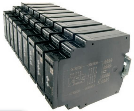
Two-hand analysis is part of the extended functionality of TELE safety relays. The S2Z021 was specially developed to analyze signals from two-hand switches, commonly used on presses. This device as well is cleared for use up to safety level 4 and as such is always the correct solution when you need to plan or upgrade machinery two-hand relays to EN 574 Type III C standards.
