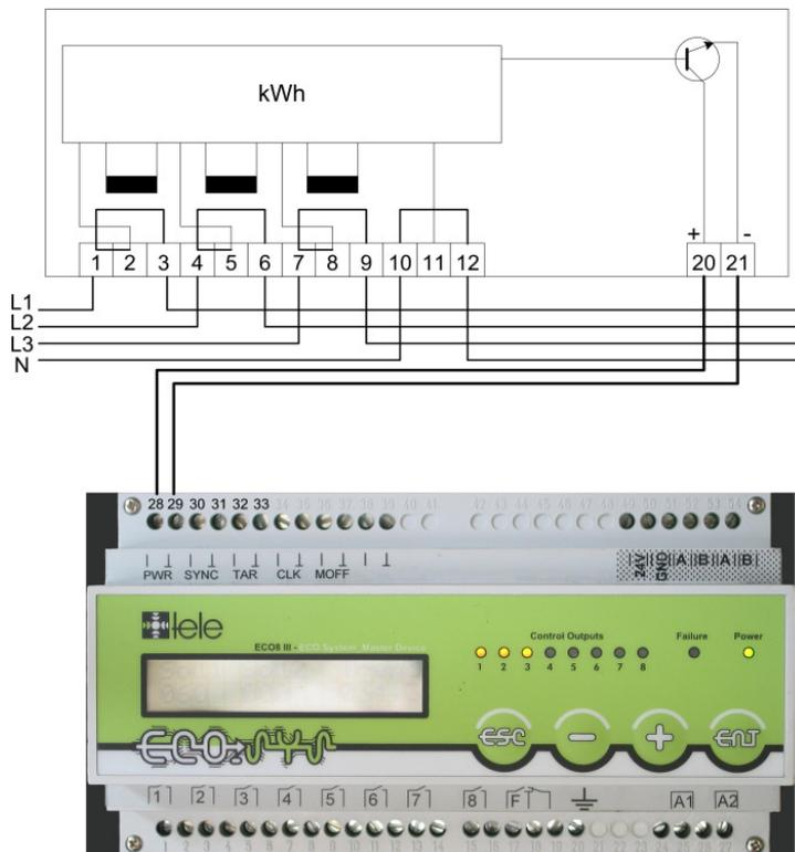
Figure 11: Connecting Diagram with Tariff Pulse
