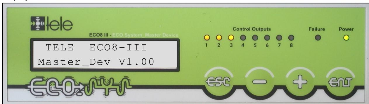
Figure 17: *ECO\_SYS* Display of the Device Information
