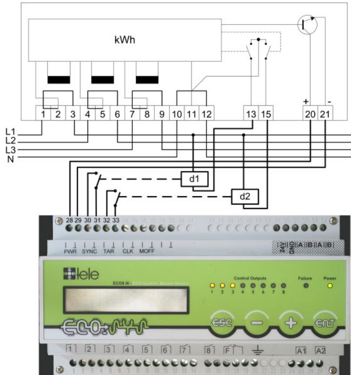
Figure 10: Connecting Diagram without Zero Potential Contacts
