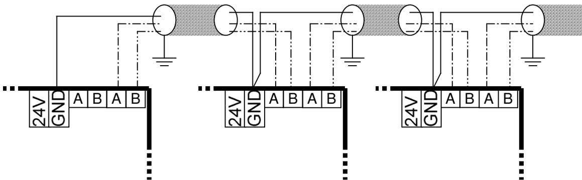
Figure 9 Bus connection with shielded cable
