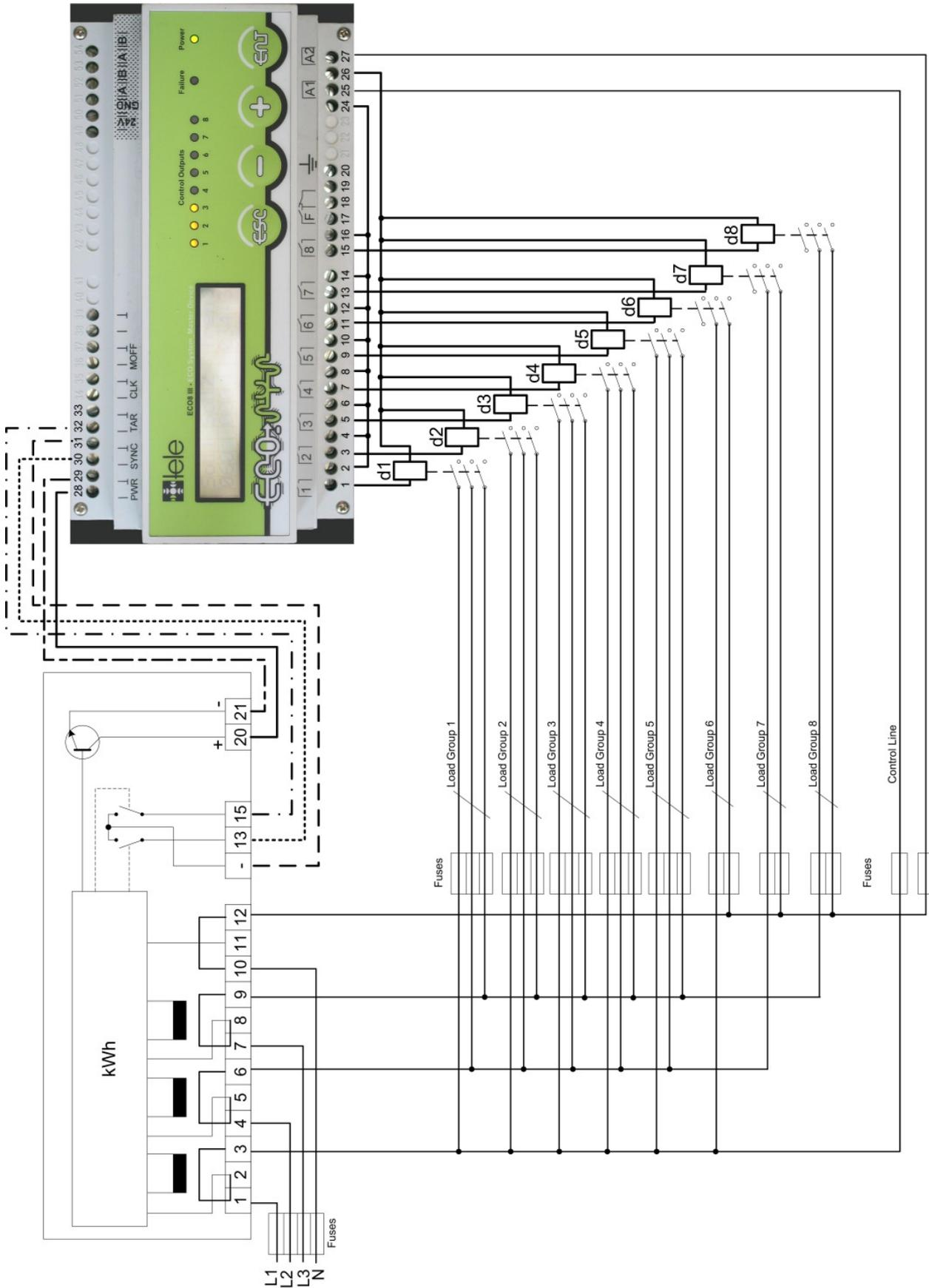
Figure 15: Wiring Scheme
