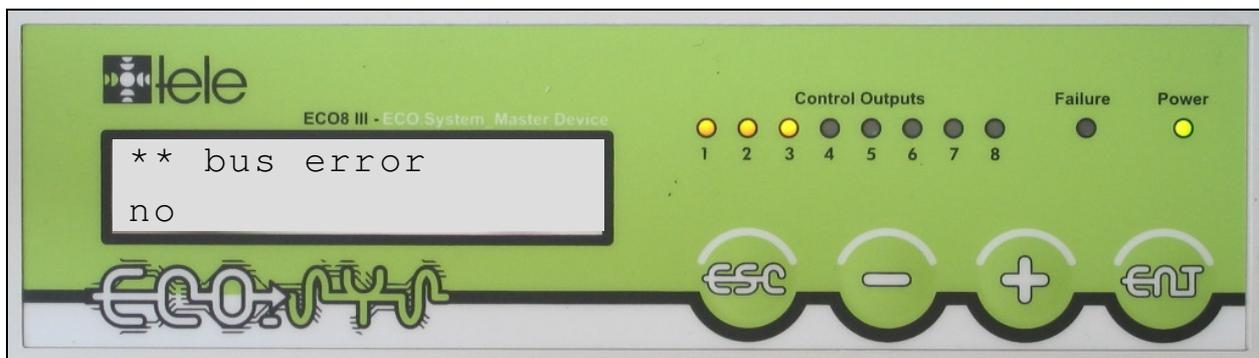
Figure 22: Display of the Bus Failure (*RS485*)
