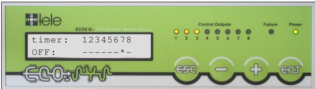
Figure 29: ECO\_SYS by Clock Timer Deactivated Outputs
