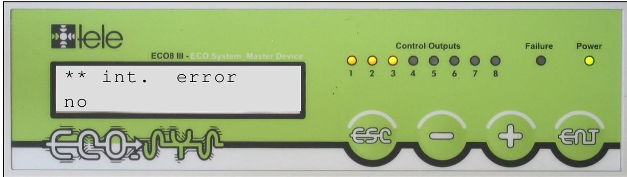
Figure 21: Display of Internal Failure
