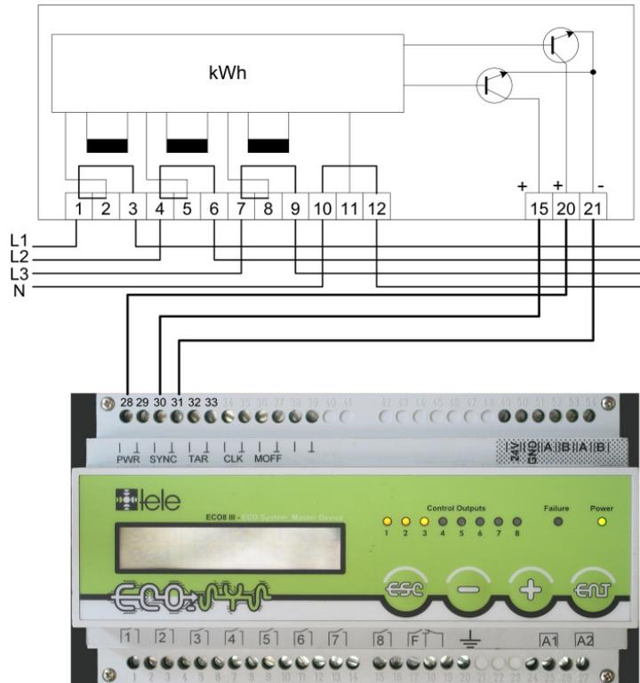
Figure 14: Connecting Diagram with a S0 Interface
