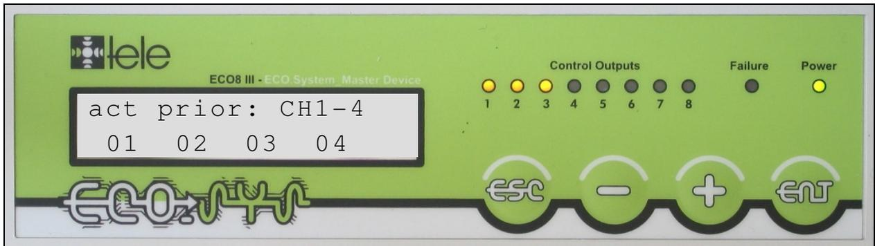
Figure 32: ECO\_SYS Current Priority Display for Channel 1 ... 4
