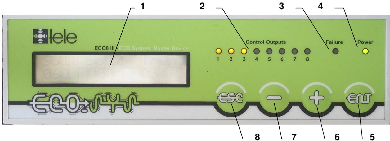
Figure 3: *ECO\_SYS* Control Elements
