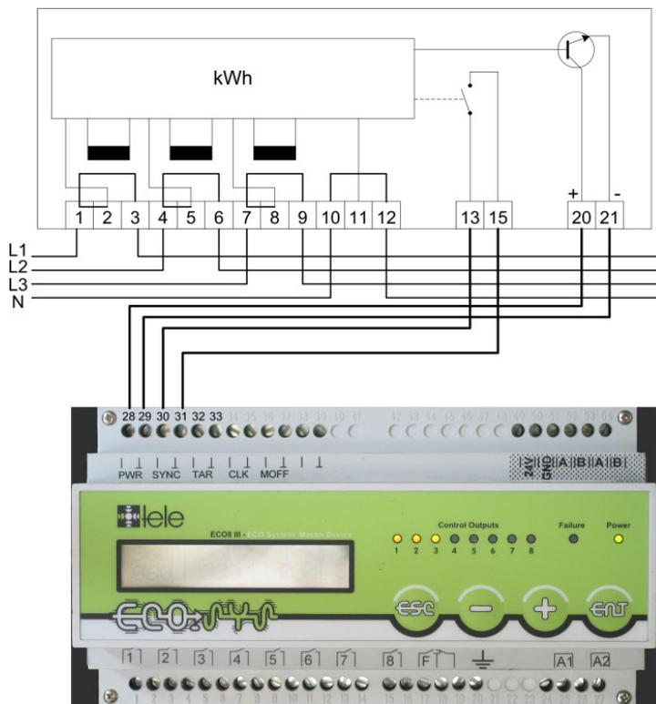
Figure 13: Connecting Diagram with Zero Potential Contacts, without Tariff Pulse
