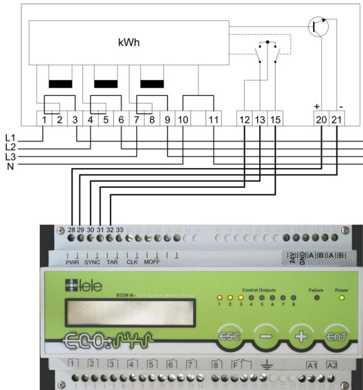
Figure 12: Connecting Diagram with Zero Potential Contacts
