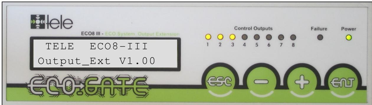
Figure 18: ECO\_GATE Display of the Device Information
