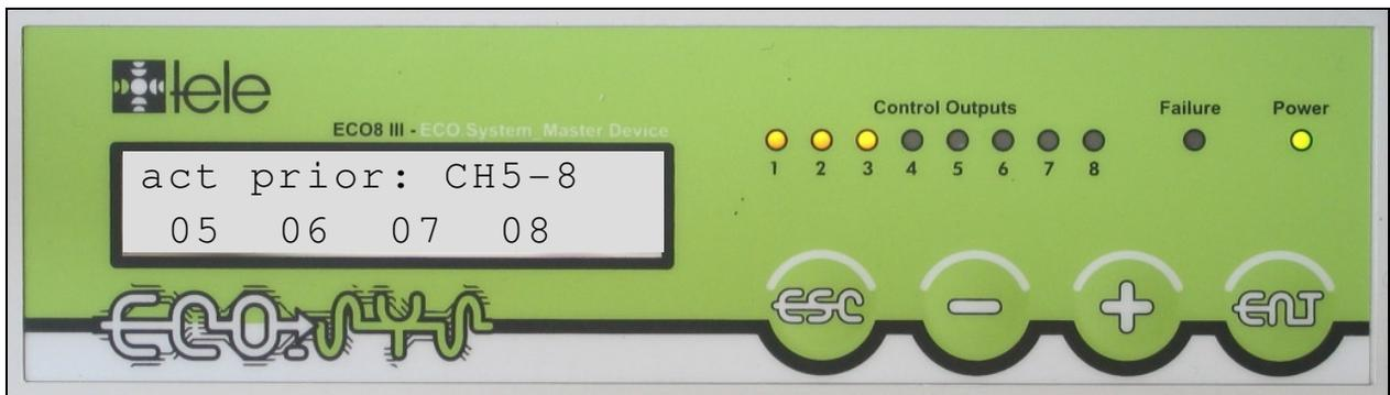
Figure 33: ECO\_SYS Current Priority Display for Channel 5 ... 8
