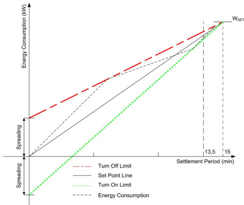
Figure 6: Integrating Load Limiter (ILL) Method
